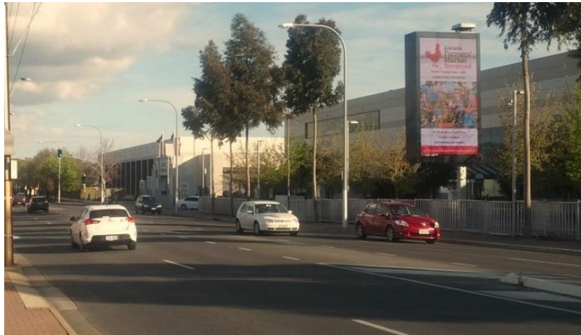
SMD in Sun-Facing Application – Washed-Out Contents
